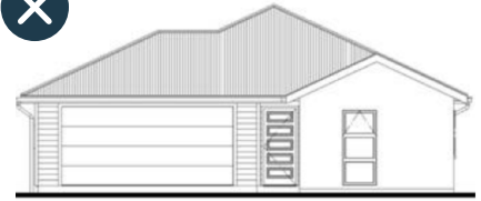
Unacceptable gable & hipped roof
